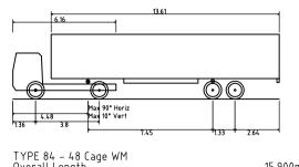
TYPE 84 - 48 Cage WM Overall Length Overall Width Overall Body Height Min Body Ground Clearance Max Track Width Lock to Lock Time Kerb to Kerb Turning Radius
