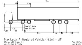
Max Legal Articulated Vehicle (16.5m) – WM Overall Length Overall Width Overall Body Height Min Body Ground Clearance Max Track Width Lock to Lock Time Kerb to Kerb Turning Radius
