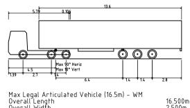
Max Legal Articulated Vehicle (16.5m) - WM Overall Length Overall Width Overall Body Height Min Body Ground Clearance Max Track Width Lock to Lock Time Kerb to Kerb Turning Radius
