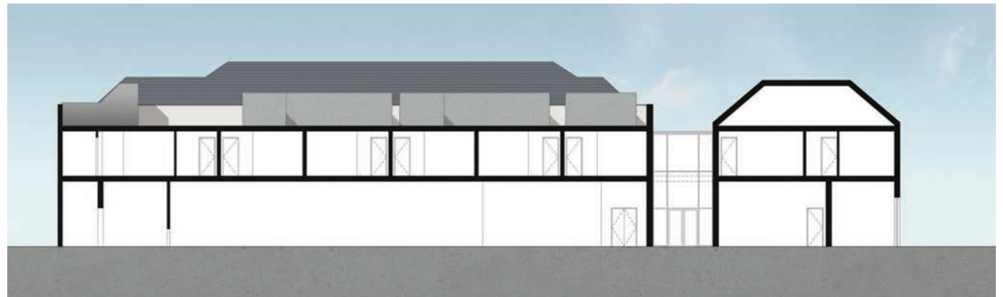
North-south section through Building 455
