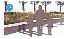
02 Timber shuttered concrete seating wall w/ polished seat surface or similar approved
