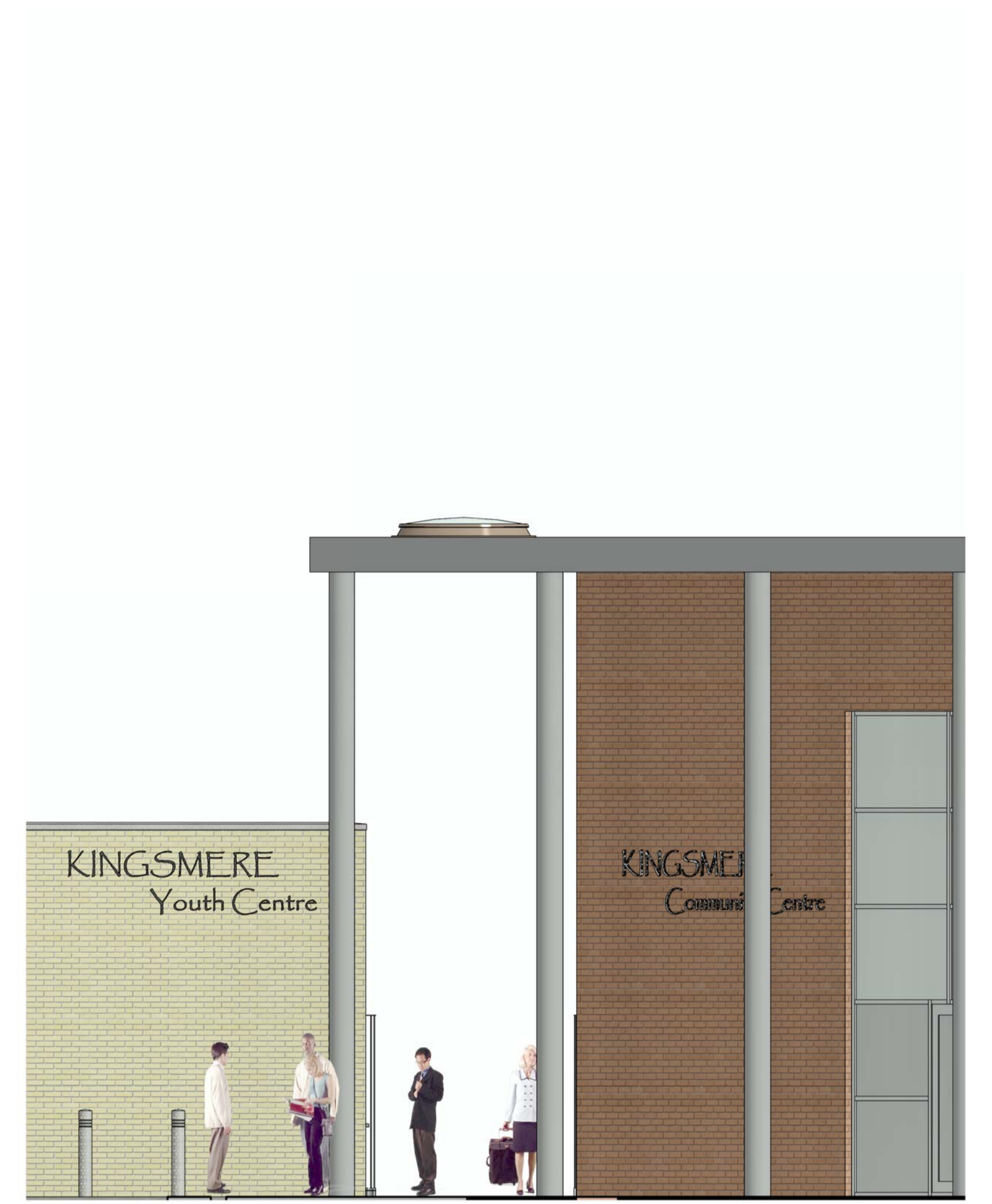
3 South West Elevation Detail 3 1 : 50
