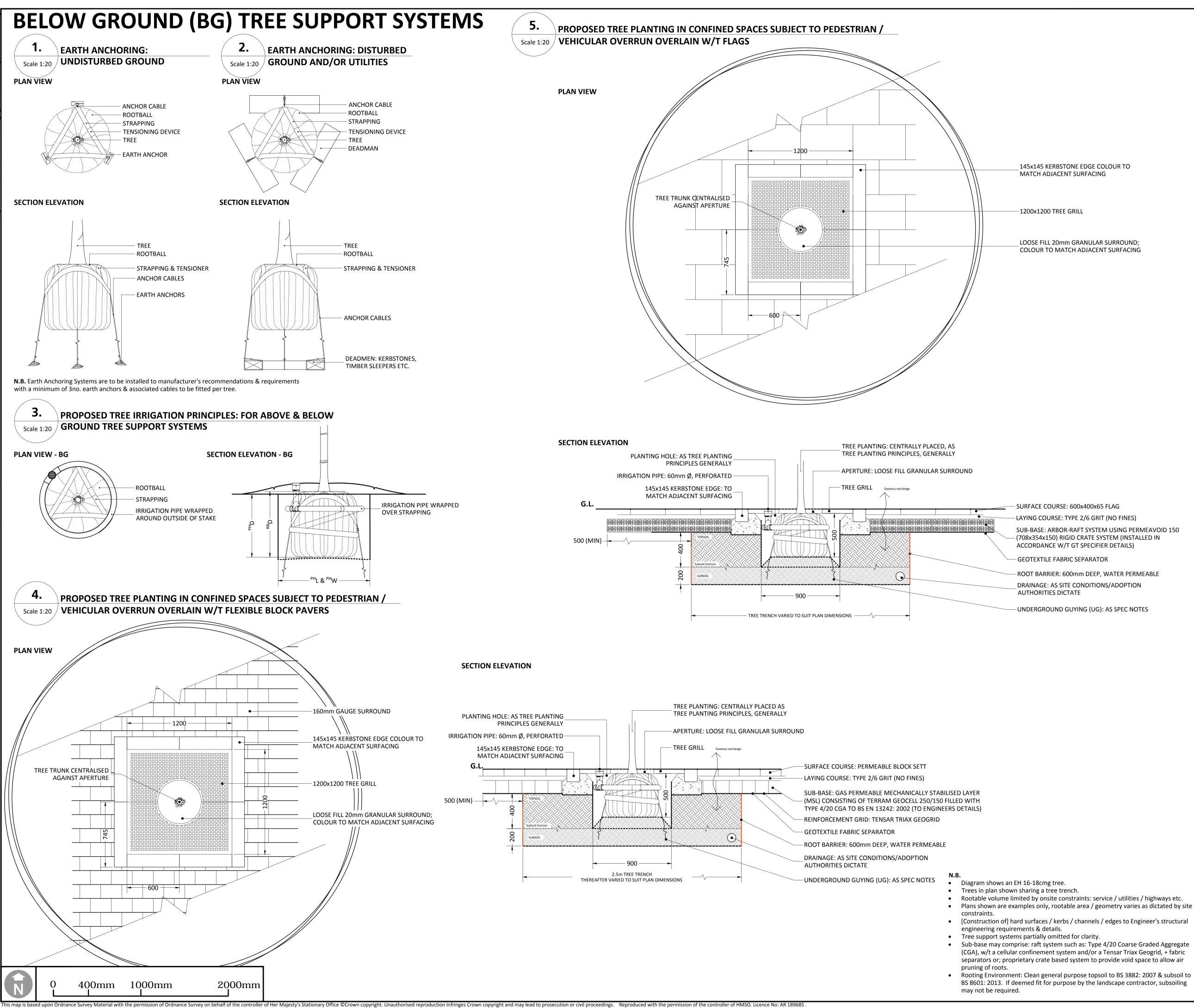
SUB-BASE: ARBOR-RAFT SYSTEM USING PERMEAVOID 150 - (708x354x150) RIGID CRATE SYSTEM (INSTALLED IN
