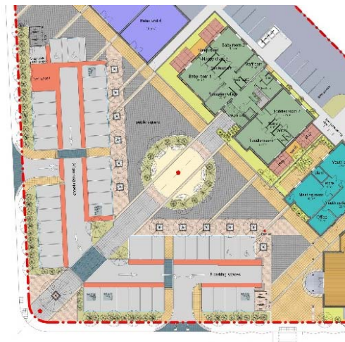
Pedestrian safety routes marked within car park area
