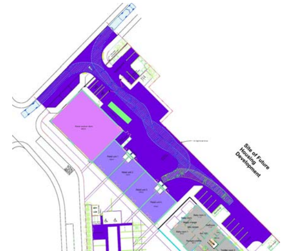
Fire tender tracking to rear service area
