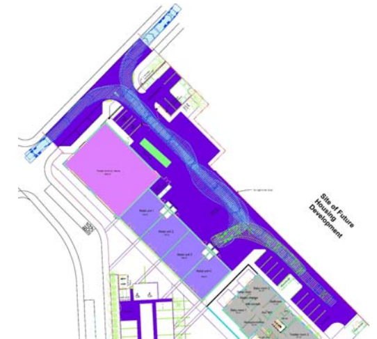
Refuse lorry tracking to rear service area
