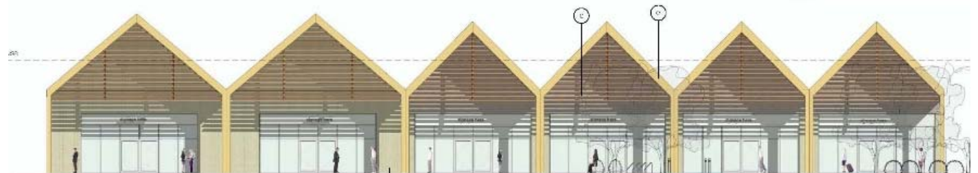
South elevation of retail area showing the variation in pitch and height
