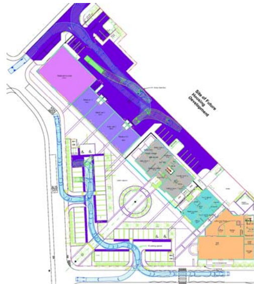
Vehicle tracking to general car parking & deliveries
