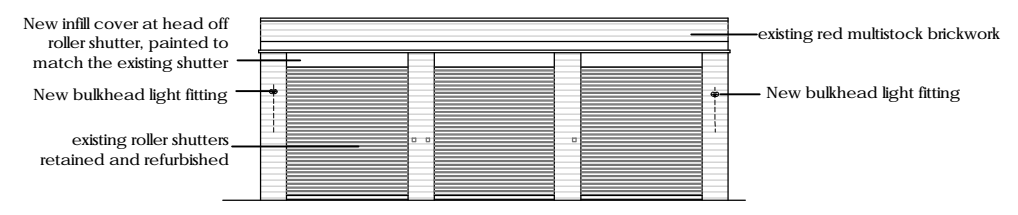
BUILDING 105 North Elevation - Proposed
