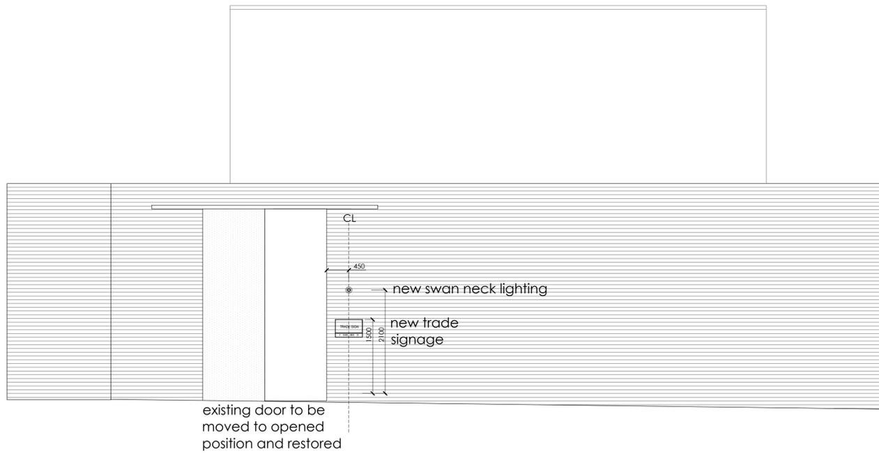
WEST ELEVATION (WITH OUTER WALL)
