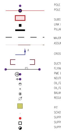
POLE MOUNTED TRANSFORMER SUBSTATION LINK BOX PILLAR MAJOR PIPELINE ASSUMED ROUTE CROSS SECTION DUCTING FLYING STAY PME EARTH NEUTRAL EARTH OIL/GAS GAUGE OIL/GAS TANK BALANCER REGULATOR SCHEMATIC CONNECTOR SUPPLY LOCATION-PROPERTY SUPPLY LOCATION-OTHER SUPPLY LOCATION-STREET FURNITURE
