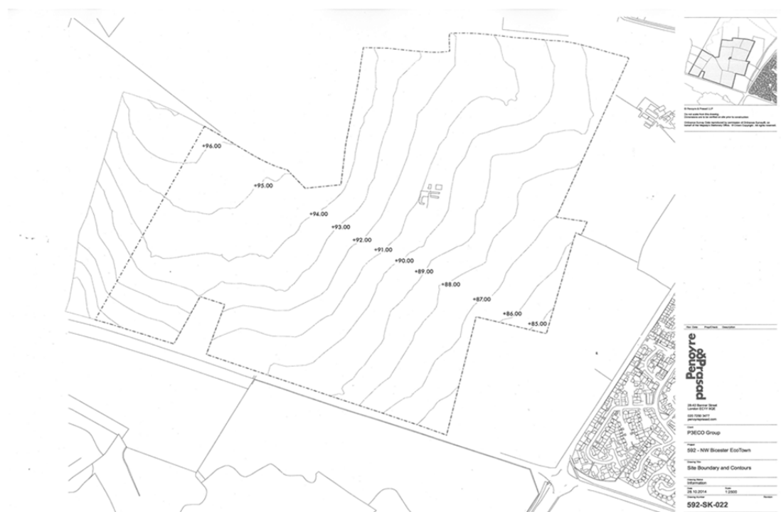
Figure 3.2 NW Bicester - Existing site topography
