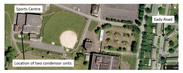
The residential properties on Eady Road are approximately 260m from the proposed plant location. Using hemispherical propagation calculations, the combined noise emissions of the plant will be approximately 20 dB.
