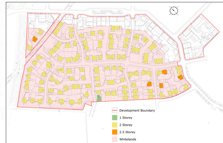
Figure 20: Proposed Layout indicating the proposed Storey Heights in the Whitelands Character Area
