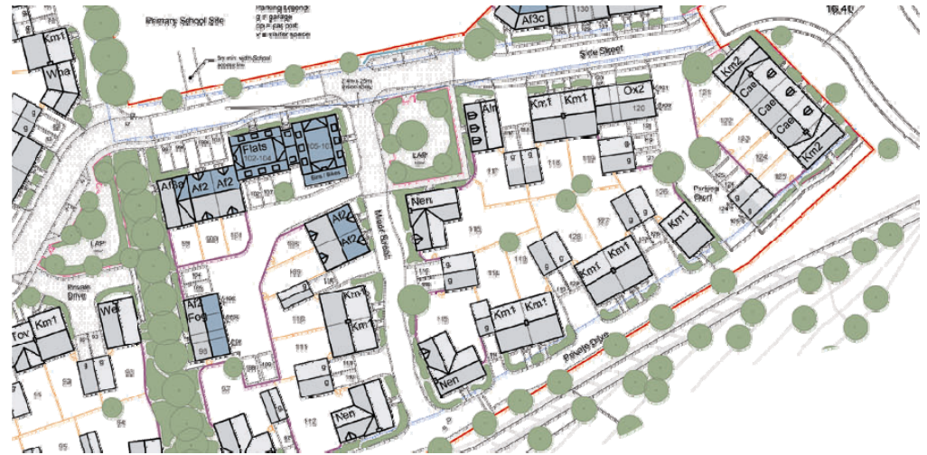
Fig.27 CAR PARKING – ILLUSTRATING ON-STREET & OFF-STREET PARKING
