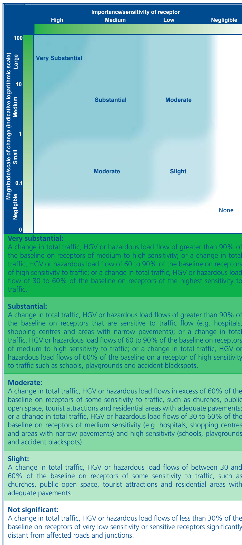
Figure 6.3 Traffic and transport significance matrix
