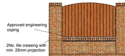
1800mm Screen Wall with Fence Infill
