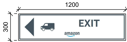
EXT07 Van Exit SIZE: 1200mm x 300mm (0.36m 2 ) QTY: 2 WALL / POLE MOUNTED HEIGHT FROM FFL: SITE SPECIFIC
