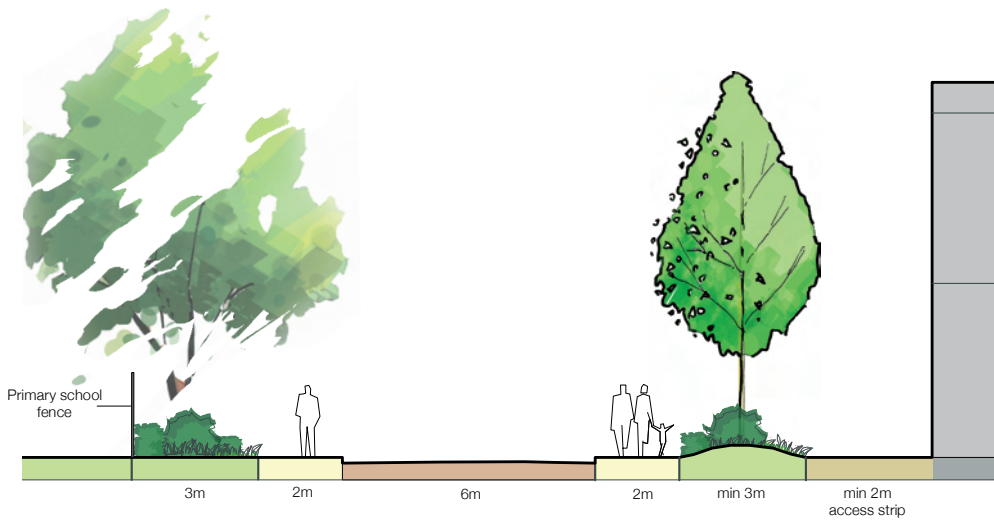
Figure 4.27 Section X-X, The minor street on the northern frontage should have a modest landscape buffer incorporating trees to soften the relationship between the Employment zone (including the Hotel) and residential uses.
