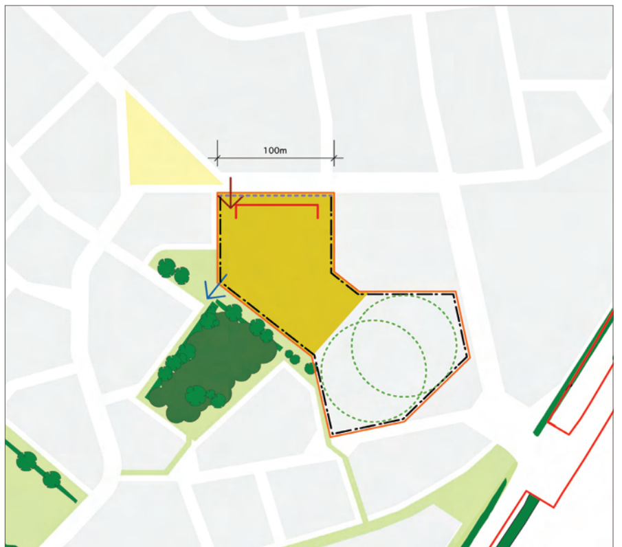
Figure 4.15 Vehicle access to the site will require an ingress on the main frontage and egress to a minor road across adopted public open space.
