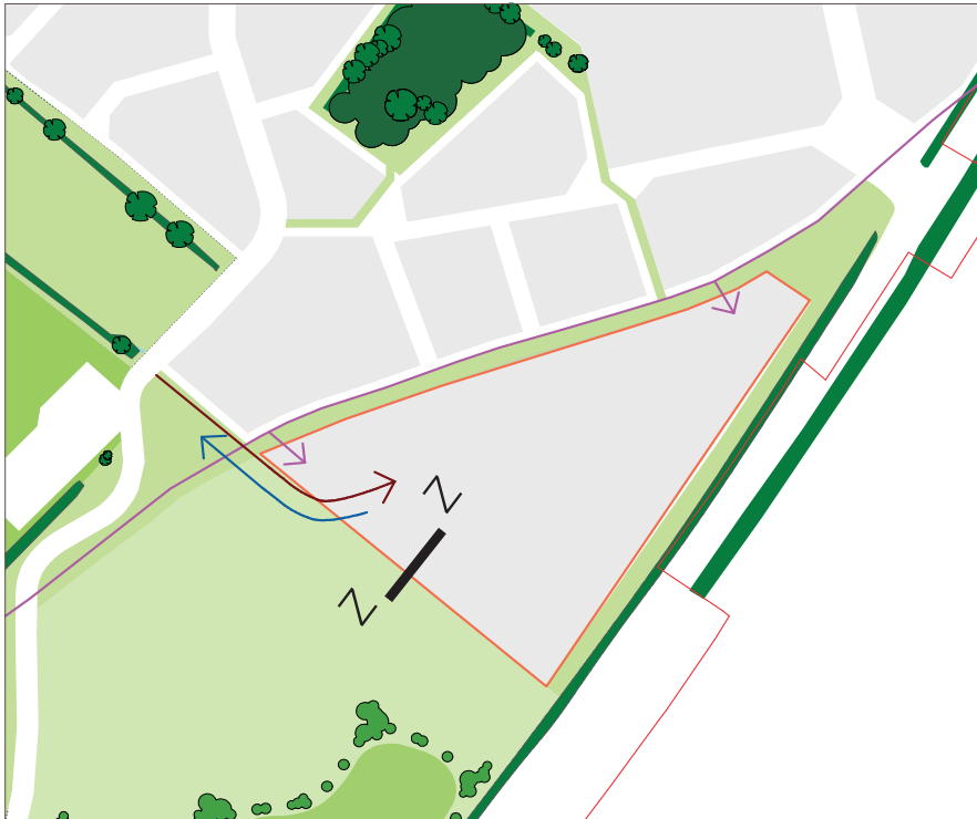
m Figure 4.18 The Education Campus will be accessed along its western boundary via footpaths, cycleways and a private drive. See figures 4.20 and 4.21 for alternative treatments for section Z-Z. See also Appendix 1, figures App1.4 and 1.5 for the Greenway and A41 frontages.
