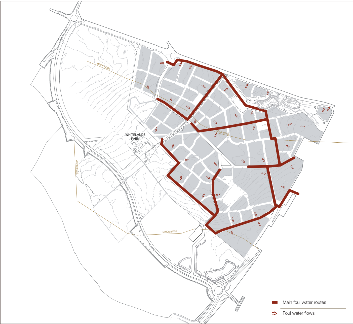
Figure 3.13 Main foul water drainage routes.
