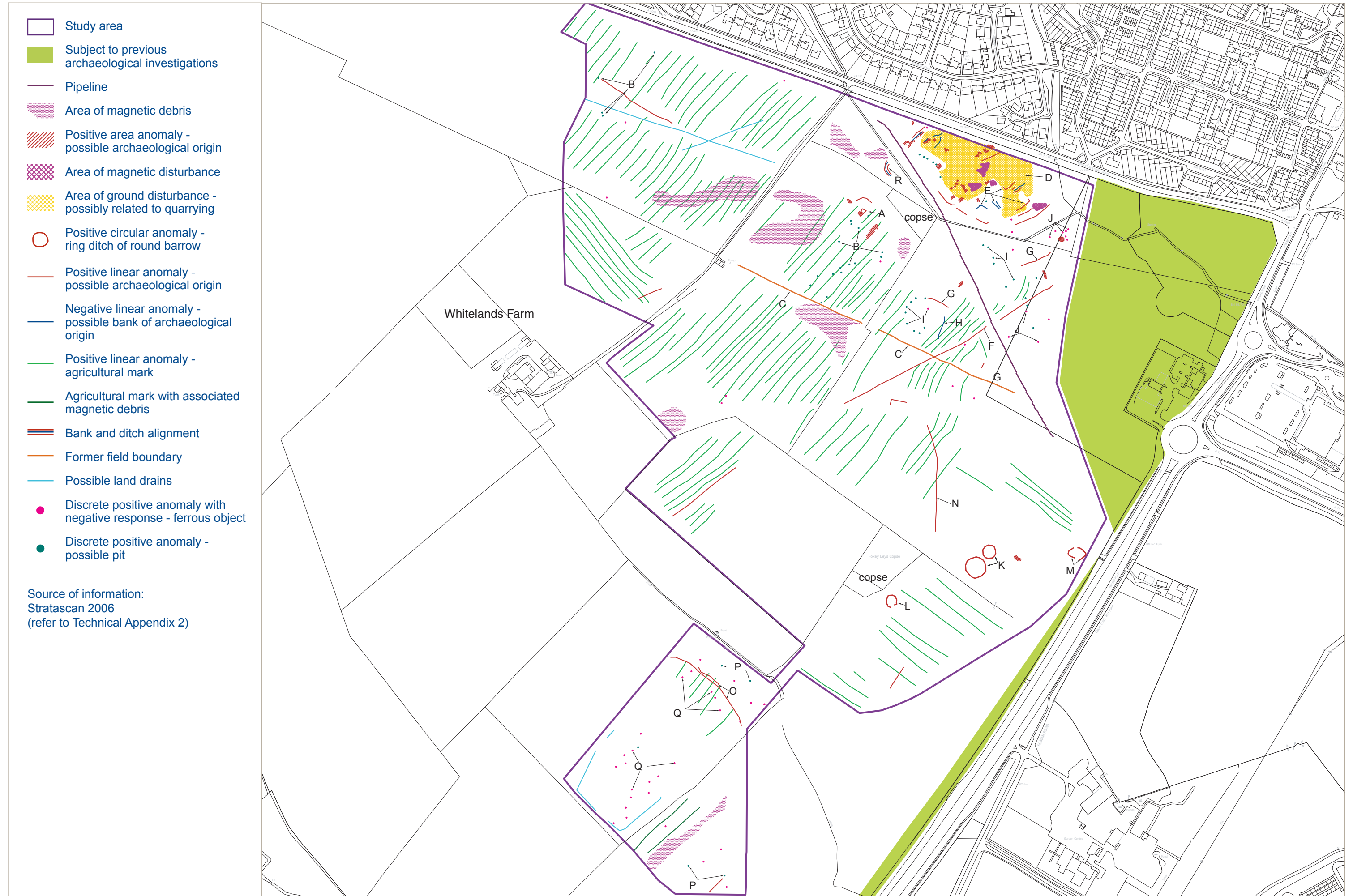
Figure 5.4 Results from the geophysical survey (after Stratascan 2006)
