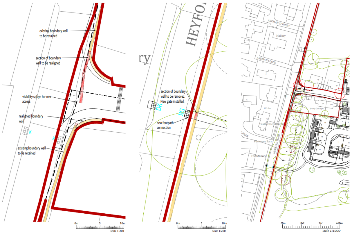
Figure 38 Plan showing proposed realignment of boundary wall, and creation of new pedestrian access.
