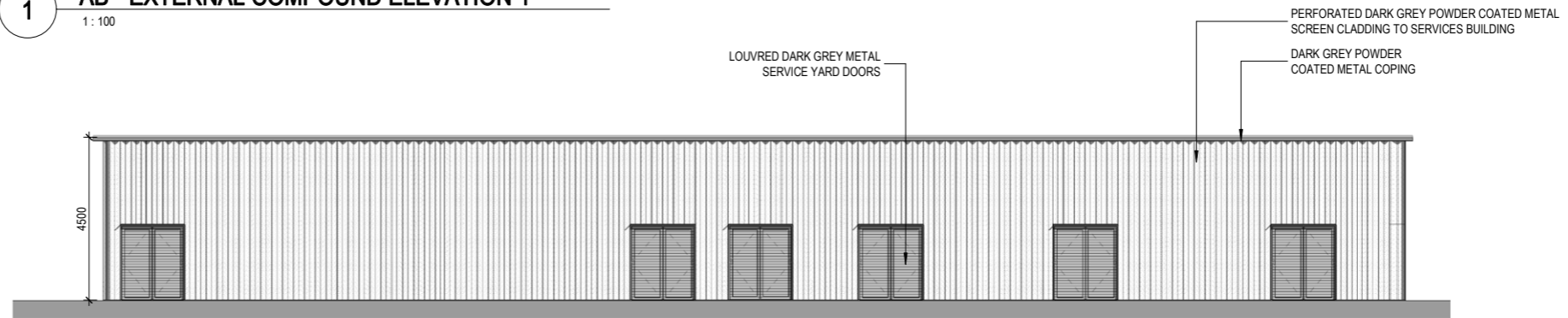
2 AB - EXTERNAL COMPOUND ELEVATION 3 1:100
