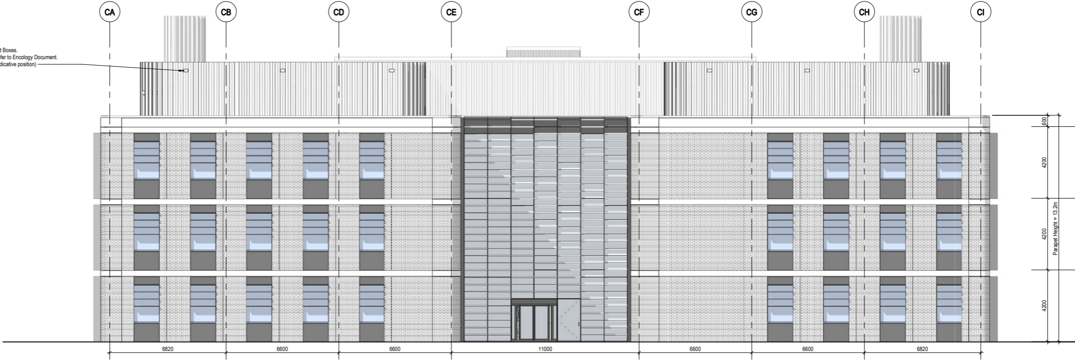
2 PROPOSED SOUTH ELEVATION - COMMERCIAL BUILDING 1:100
