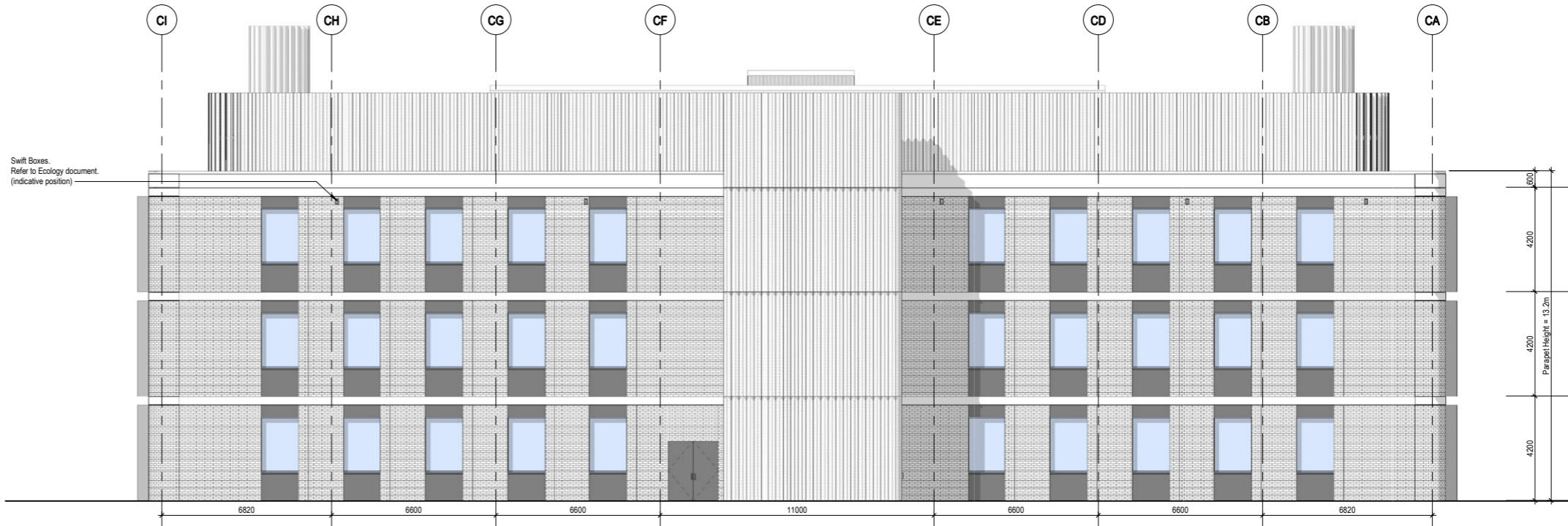
1 PROPOSED NORTH ELEVATION - COMMERCIAL BUILDING 1:100
