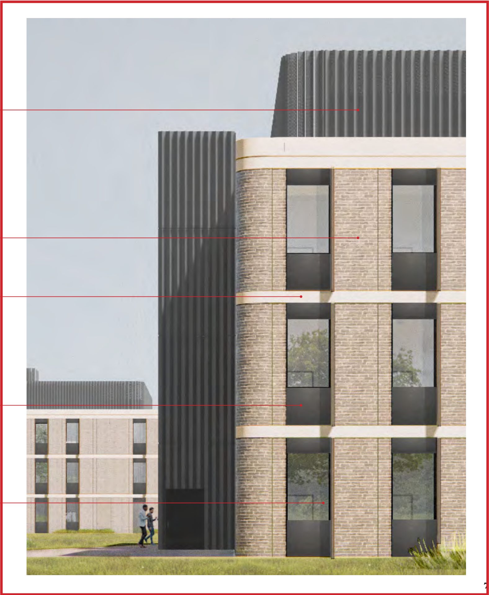
Plant Screen Panels: perforated undulated PPC metal - dark grey colour
