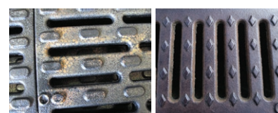
Images showing stages in the process of patination. The period of oxidation depends on the environmental conditions. Photo on the right shows a stable buffed grate
