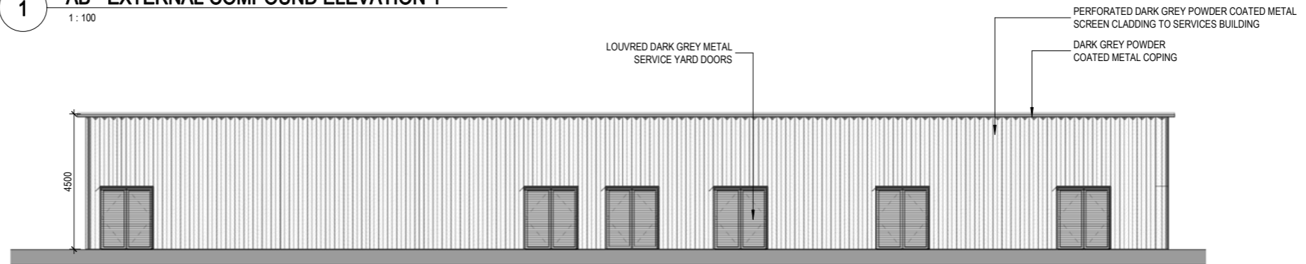
2 AB - EXTERNAL COMPOUND ELEVATION 3 1:100
