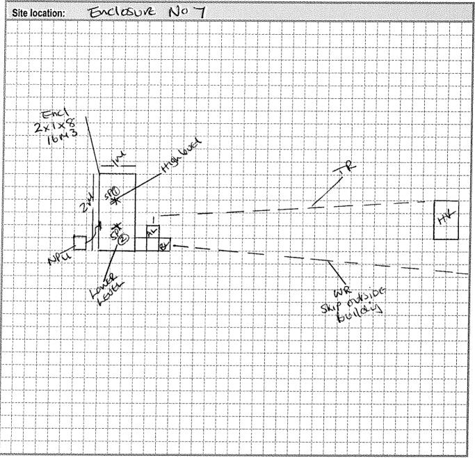
Main work area features agreed with and signed by the asbestos removal contractor's representative and ace technician
