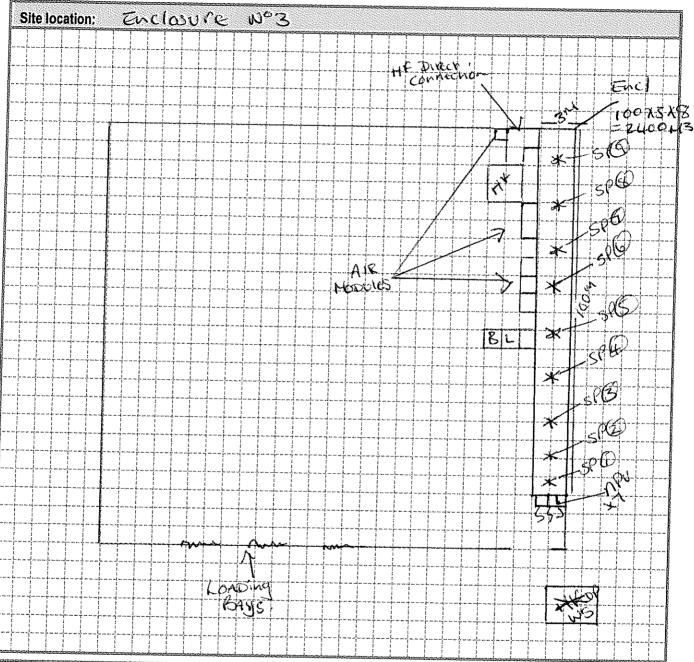
Main work area features agreed with and signed by the asbestos removal contractor's representative and ace technician Technician's name: Contractor's name: PEUENLEY. Signature: Signature: KEY: Enclosure Waste skip WS Negative pressure unit NPU Work area WA Airlock
