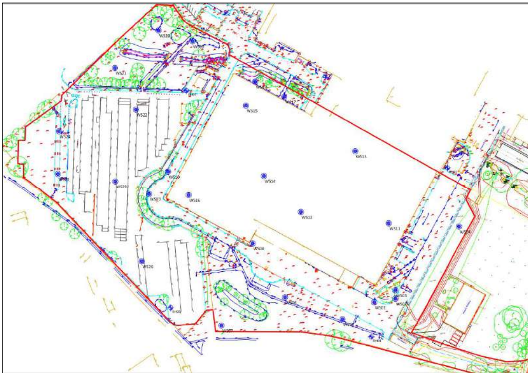
Figure 2 – Hydrock Intrusive Exploratory Locations across Site
