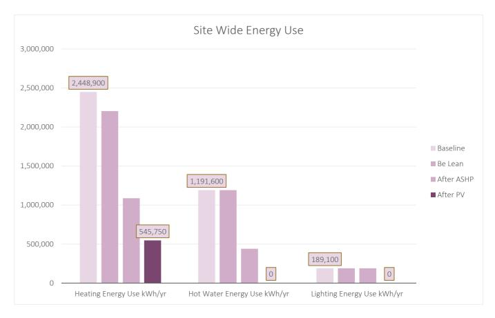
Figure 12 - Site wide energy use after PV (for this calculation PV is assumed to offset lighting, domestic hot water and 50% of the heating demand)
