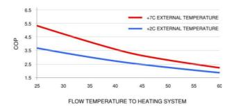
Figure 8: COP as a function of flow temperature for typical ASHP
