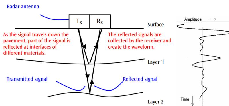
Figure 3 Example of Radar Signals at Pavement Interfaces
