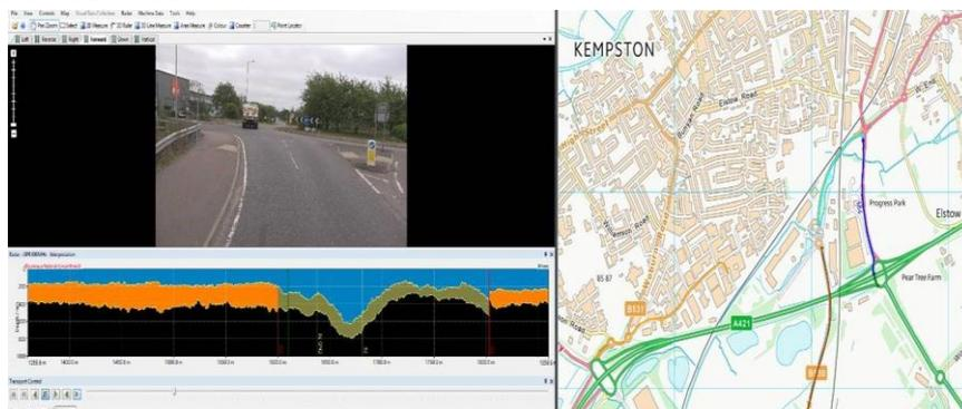
**Figure 6 Example of Data Processing Software "Roadshow"**
