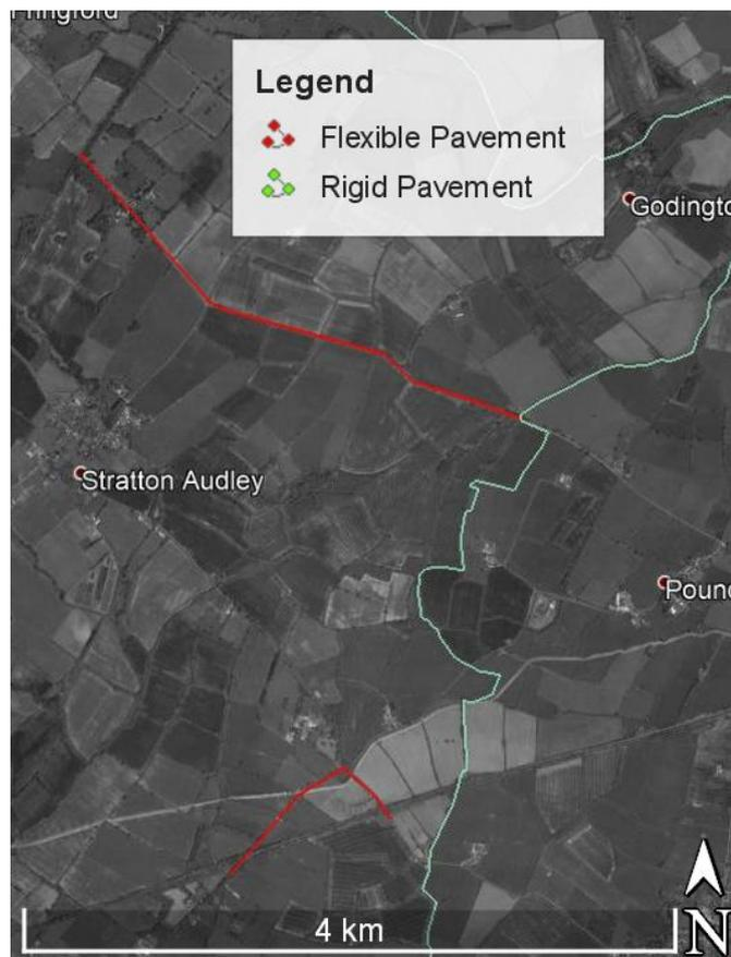
**Figure 8 Pavement Type Identified from GPR Data**
