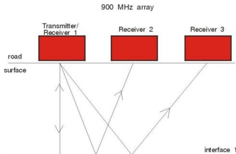
**Figure 5 Auto-Calibration Method: Common Depth Point (CDP)**
