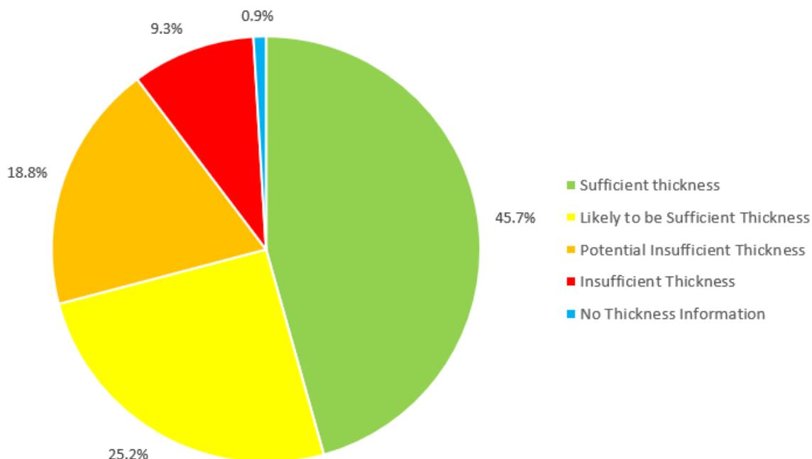
**Figure 9 Pavement Thickness Range Identified from GPR Data**
