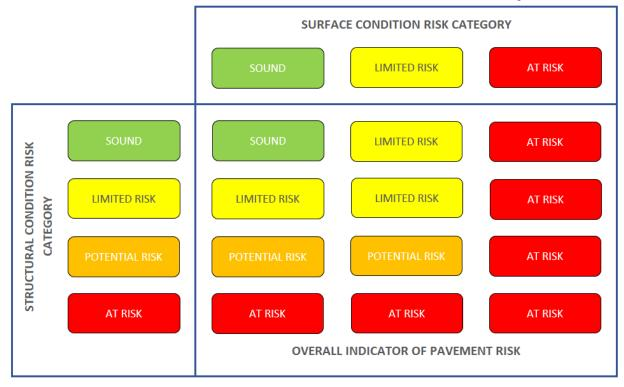
Figure 7 Calculation of Overall Indicator of Pavement Risk
