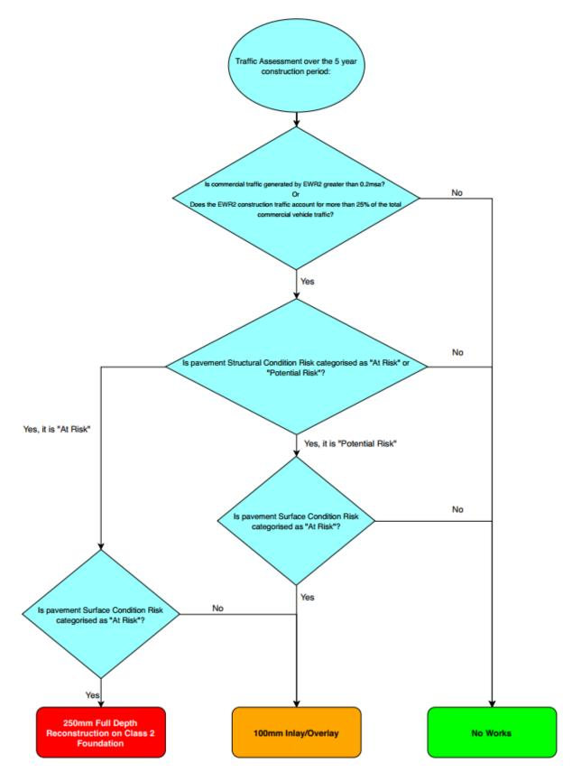
Figure 15 Pavement Treatment Methodology for Stages 1 & 2
