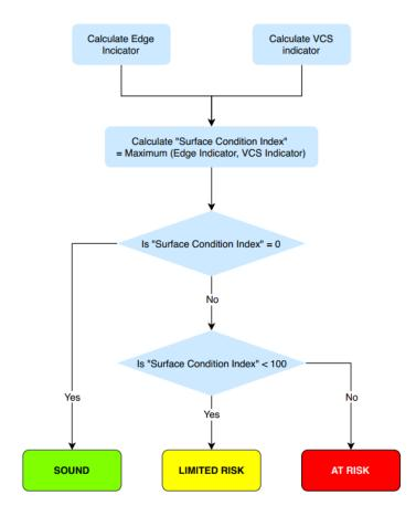
Figure C-17 Calculation of Overall Indicator of Pavement Risk
