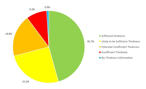
Figure 9 Pavement Thickness Range Identified from GPR Data
