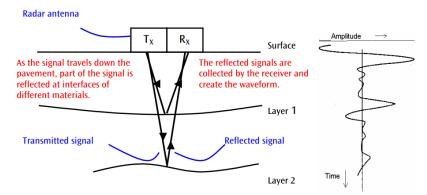
Figure 3 Example of Radar Signals at Pavement Interfaces
