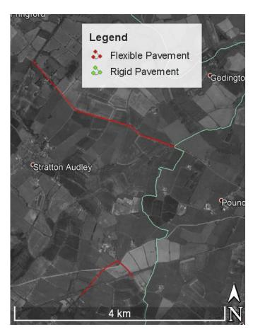
Figure 8 Pavement Type Identified from GPR Data
