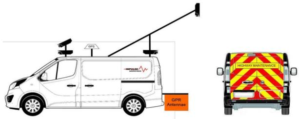
Figure 4 Impulse Geophysics Survey Vehicle
