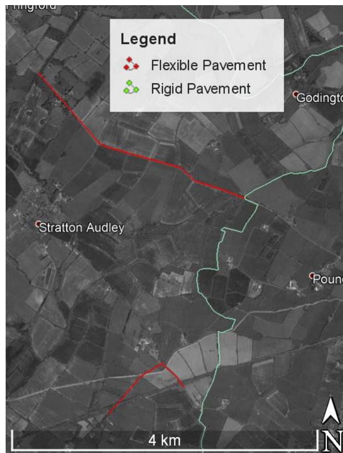
Figure 8 Pavement Type Identified from GPR Data
